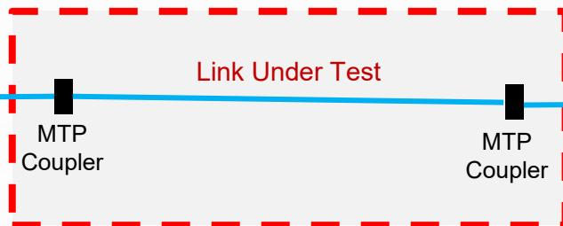
*Loss measured is of all components in box:*
